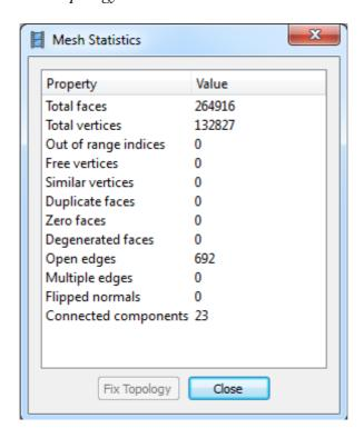
PhotoScan tends to produce 3D models with excessive geometry resolution. That's why it is recommended to decimate mesh before exporting it to a different editing tool to avoid performance decrease of the external program.
