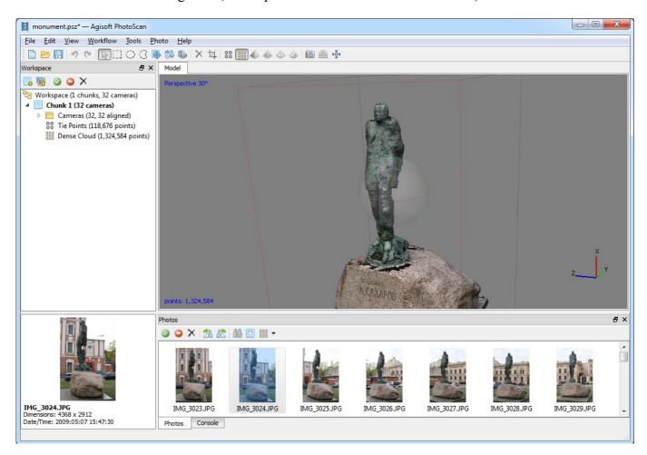
Points from the dense cloud can be removed with the help of selection tools and *Delete/Crop* instruments located on the Toolbar.
