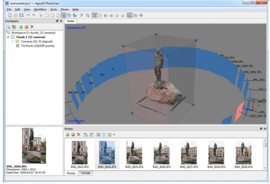
This step is optional since PhotoScan automatically calculates bounding box dimensions and location. But it is recommended to check if any correction is needed, because geometry reconstruction step deals only with the point cloud inside the volume.
