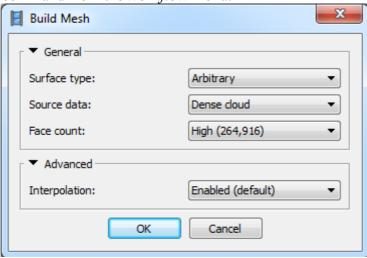
Set the following recommended values for the parameters in the *Build Mesh* dialog:
