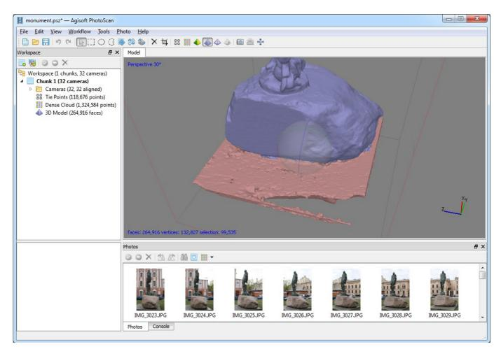
In some cases building geometry without interpolation may result in small non-connected with the main model components generation. To ease the selection and removal of such components you can use *Gradual Selection* command from the *Edit* menu.
