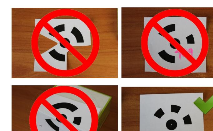
Once the coded targets are printed, place them in the scene or around the object of interest so that they could be clearly seen from at least of couple or images.
